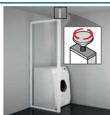
Perfil a techo / Ceiling profile
